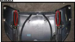
The rods on which the electric windscreen travels should be cleaned and lubricated annually. This reduces the load on the windscreen motor and will prolong its service life. BMW recommends using a silicone lubricant as that tends to attract less dust than other lubricants. I use this:
