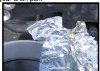
Note: Before changing any oil always remove the filler plug first. The last thing you want is to drain it and then not be able to refill it. This is seldom an issue on K bikes though.
