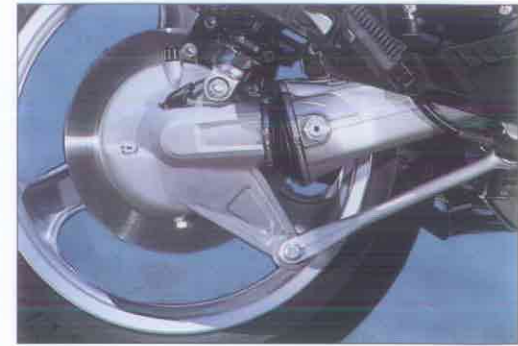
Suspension technology at its very best: The patented BMW Paralever reduces load change responses and brake stutter, and improves riding comfort, traction and handling especially in fast bends and on rough surfaces.
